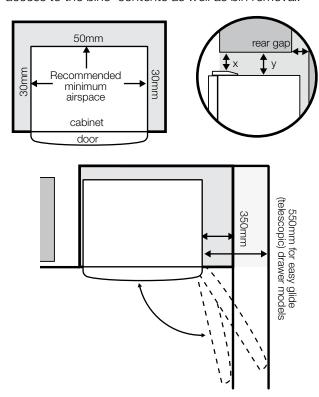
NOTE: Doors are designed to sit proud of cabinetry (not flush). The clearances shown above are the recommended minimum clearances.
